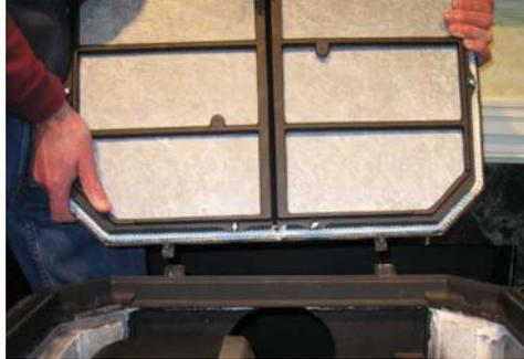
20. Once the repair is complete, you may fire up your stove right away, however, we recommend that you recheck the furnace cement seal after 2-3 days of burning and add cement if necessary due to shrinkage.
