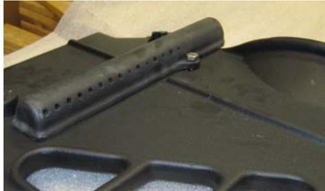
*Note: Certain models will not have a secondary air tube. Check the flue collar located at the rear of the stove. If you do not have a 3/4" diameter hole in the bottom left hand corner of your flue collar then you do not have a secondary air tube.*
