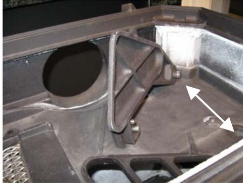
16. Install the combustor so that the stainless divider faces the left wall.
