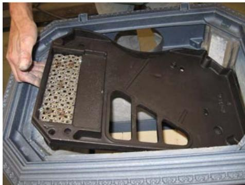
11. Insert new 5/16" gasket along the perimeter of the baffle and then apply a bead of furnace cement over it. Use your fingertip (you may want to put a piece of plastic wrap over your finger first) to press the cement firmly into the seam and leave a smooth finished look.
