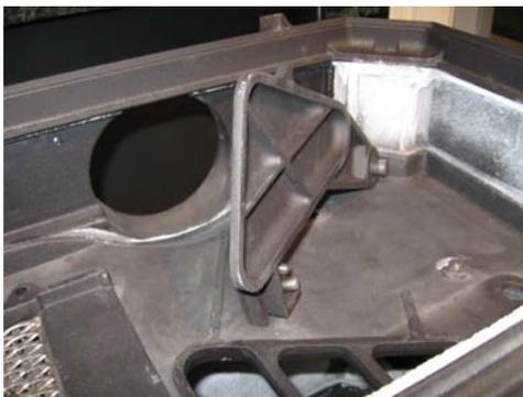
6. Remove the secondary air tube from the firebox side of the baffle by holding the bolt in the firebox with a wrench and turning the nut on the top side of the baffle with a socket and lower the tube off the baffle (Alternately, you can do this step after you have completely removed the old baffle).
